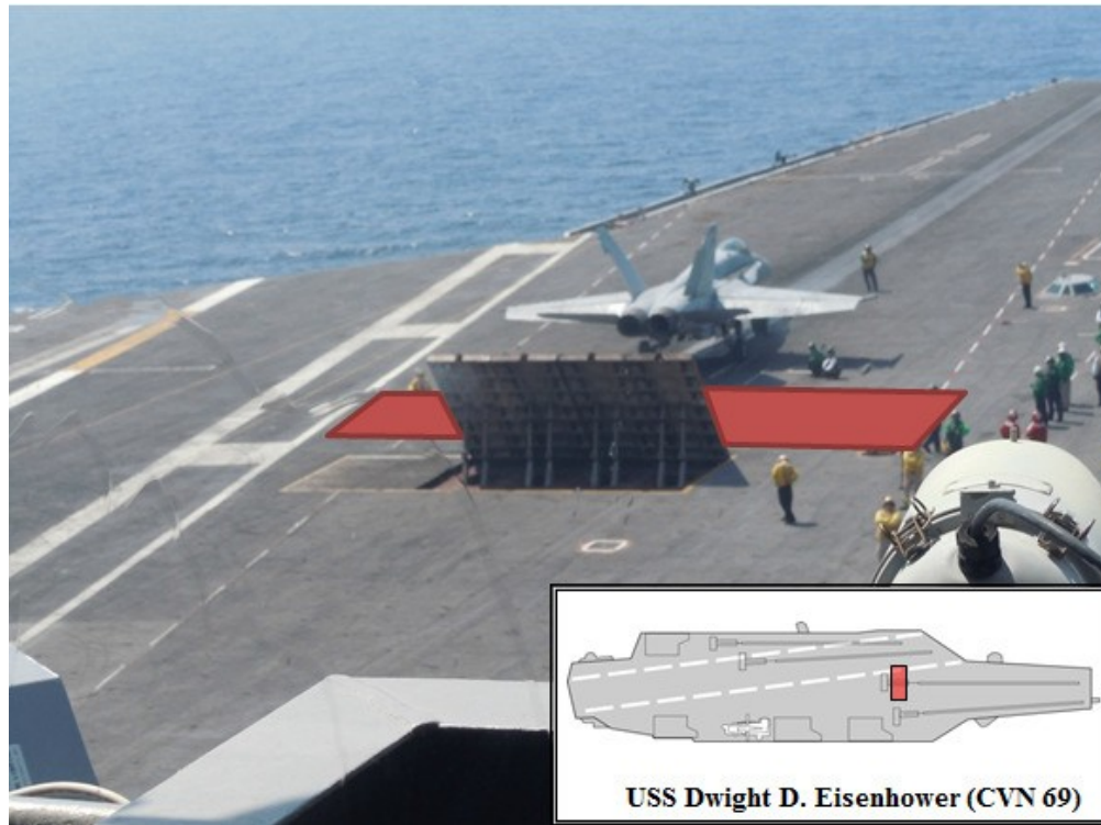
Figure 2. Location relative to flight deck operations of damping treatment and measurement location focus
