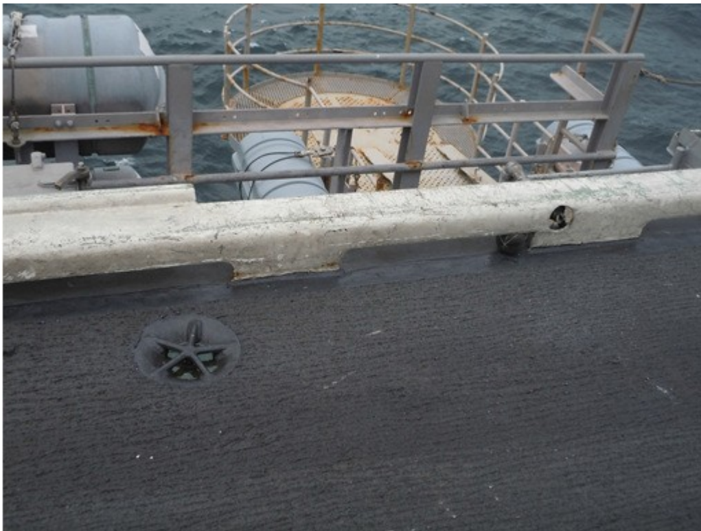
Figure 11. Microphone installation on flight deck envelope
