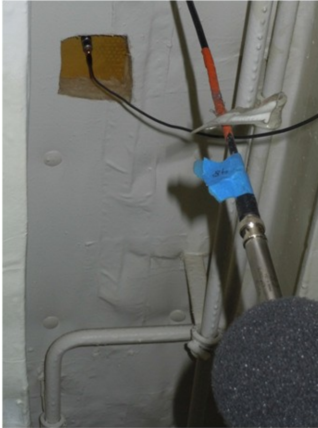
Figure 6. Accelerometer installation on flight deck underside
