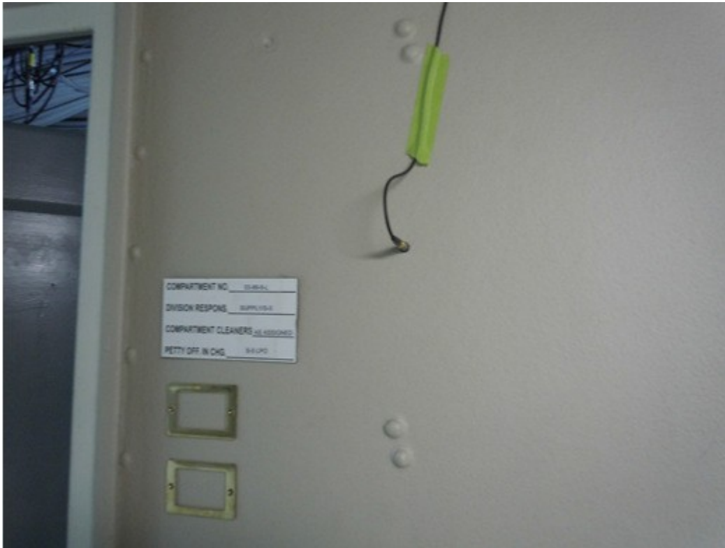
Figure 8. Accelerometer installation on joiner bulkhead
