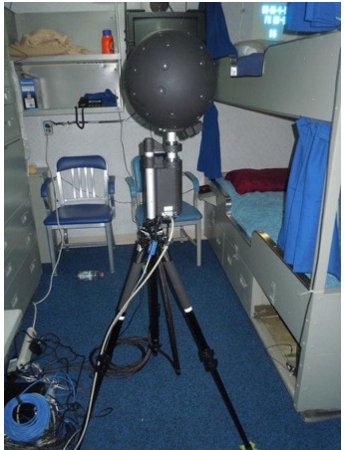
Figure 13. LMS spherical acoustic array used to determine "hot spot" locations where acoustical energy is entering compartments
