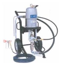
GRACO 33:1 OR 41:1 AIR OPERATED AIRLESS SPRAY UNITS AS WELL AS THE OLDER 28:1 UNITS WORK WELL WITH TEMP-COAT® APPLICATIONS. USE 18 TO 21/1000 TIPS WITH #5 OR #6 FAN.Graco 28:1, 2300 PSI, 3 GPM Airless Pump OR ANY OTHER MANUFACTURERS PUMP MEETING THESE SPECIFICATIONS SHOULD PERFORM WELL WITH TEMP-COAT® (SEE REVERSE SIDE FOR OTHER SPECIFICATIONS)
