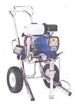
GRACO 7900 GAS OPERATED AIRLESS PUMP THIS IS A MASTIC TYPE PUMP DESIGNED FOR HEAVY FLUID APPLICATION. SIMILAR EQUIPMENT MAY BE AVAILABLE FROM OTHER MANUFACTURERS. USE 18 TO 21/1000 TIPS WITH #5 OR #6 FAN. THE GRACO PLUS GUN OR CONTRACTORS GUN WORKS WELL WITH OUR PRODUCT.
